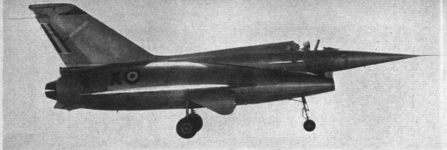
First prototype Nord 1500 Griffon canard (tail-first) delta-wing, missile-armed interceptor. The power unit is a S.N.E.C.M.A. Atar 101E.
