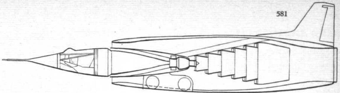
**Leduc 022.** Supersonic aircraft with integral ramjet. The body forms the duct for a supersonic ramjet, suitable for Mach numbers in excess of 2.0. In the centre is mounted an Atar 101 F turbojet with afterburner, which provides starting thrust and drives accessories. There are six concentric flameholders. Maximum thrust is estimated at 140,000 lb. This aircraft may fly at the end of this year.
