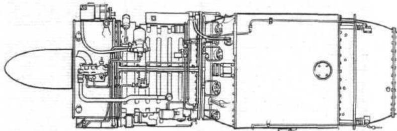
**S.N.E.C.M.A. R.105 Vesta.** Single-shaft turbojet. Seven-stage compressor, annular combustion chamber with ten burners and single-stage turbine. Diameter, 26.8in; length as shown, 78.7in; dry weight, 639 lb; mass flow, about 50 lb/sec; pressure ratio, about 5.5:1; maximum thrust, 3,085 lb, type tested, at 11,000 r.p.m. with s.f.c. of 0.99. An afterburning version of the Vesta has been developed.
