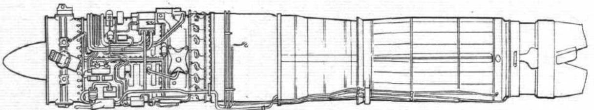
**S.N.E.C.M.A. Atar 101 F-2.** Turbojet with afterburner. Seven-stage compressor, annular combustion chamber and single-stage turbine; afterburner to reheat to about 1,900 deg K. Overall diameter 36.2in; length, 227.8in; dry weight, 2,557 lb; mass flow, 110-112 lb/sec; pressure ratio, 4.52:1; maximum thrust, 8,370 lb at 8,300 r.p.m. with s.f.c. of 2.0 (without afterburning, about 6,500 lb with s.f.c. of 1.02).
