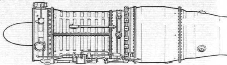
**S.N.E.C.M.A. Atar 8.** Turbojet. Nine-stage compressor, annular combustion chamber and (probably) two-stage turbine. Diameter, 36.2in; length, about 130in as shown; dry weight, about 2,100 lb; mass flow, about 140 lb/sec; pressure ratio, about 7:1; maximum thrust, 9,255 lb at 8,400 r.p.m. with s.f.c. of about 0.93.
