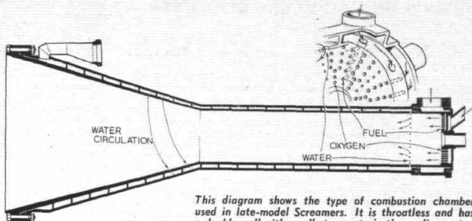
*This diagram shows the type of combustion chamber used in late-model Screamers. It is throatless and has a double wall with scrolls to constrain the cooling water.*
