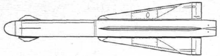
**Falcon 1.** AAM with 6,000 lb-thrust solid-propellant motor; no boost motor. Length, 6ft 6in; span, 2ft 6in (reduced to 1ft 6in in a later variant); body diameter 6in; weight, 112-122 lb; burn-out speed,  $M=2.8$ ; operational range, 4 miles.
