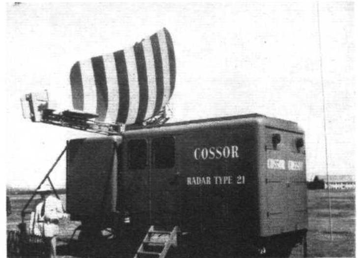
In operation at Blackbushe during M.T.C.A. trials; the Cossor CR.21 surveillance radar in its mobile version.
