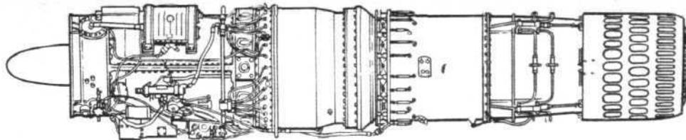
**Wright J65-W-6.** Single-shaft turbojet with afterburner. Thirteen-stage compressor, annular combustion chamber with 36 vaporizing burners and two-stage turbine. Diameter, 37.9in; length, 195in; dry weight, 2,780 lb; mass flow, 120 lb/sec; pressure ratio, 7:1; maximum thrust, 11,200 lb with reheat, at 8,200 r.p.m., with s.f.c. of 1.97. The basic engine has a dry rating of 7,800 lb thrust with s.f.c. of 0.91.
