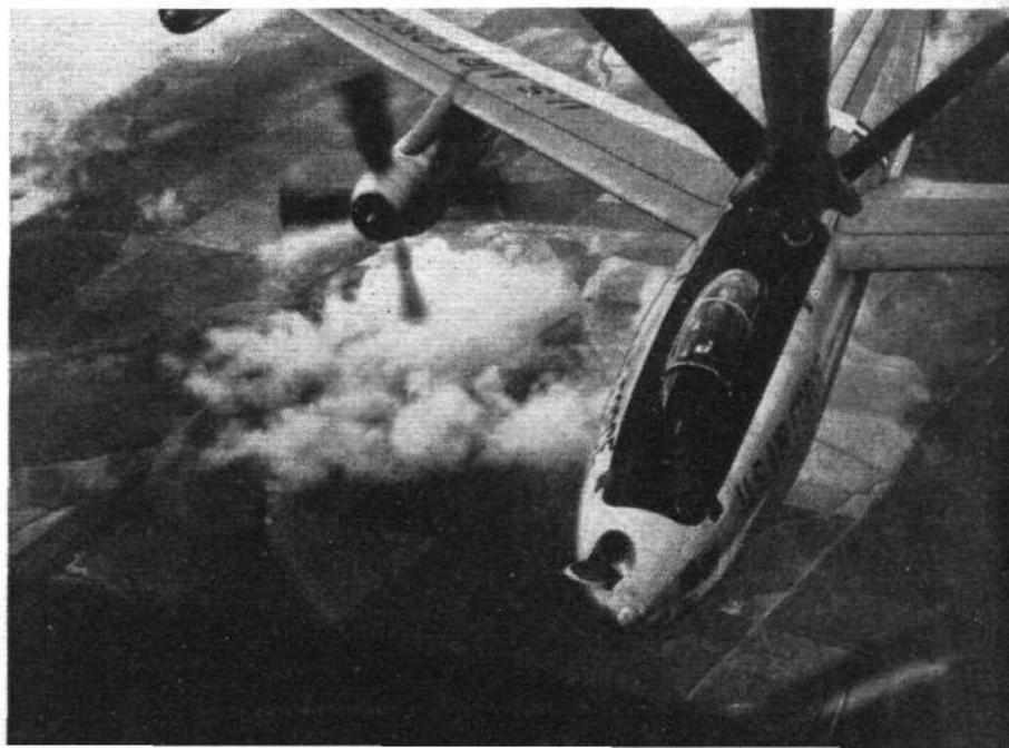
During 1956 the two XB-47D test-bed aircraft flew many hours with the Wright T49 turboprop. Here one is seen from a KC-97 tanker.
