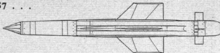
**de Havilland Propellers Firestreak (Blue Jay)** Air-to-air. Solid sustainer motor. Length, 10ft 5.28in; body diameter, 8.67in; span of wings, 29.4in; span of controls, 19.1in. Weights and performance data restricted.
