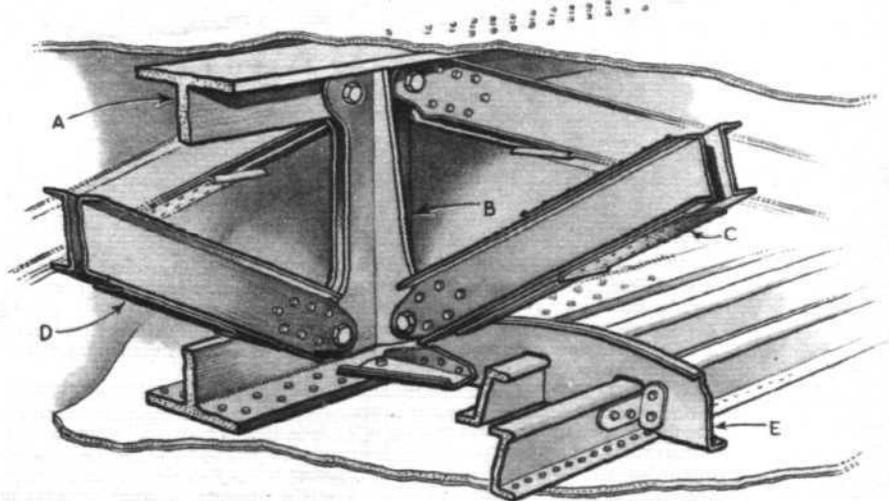
Above is a detail showing the general type of interior structure employed between the wing skins. A, spar boom; B, vertical post; C, diagonal rib bracing; D, diagonal spar bracing; E, under-surface rib former.
