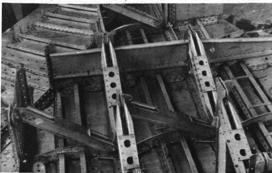
On the left is a photograph of a portion of the bottom skin adjacent to the root, showing the interior structure being assembled thereon. The light-coloured area at the upper left lies within the fuselage and terminates at the aircraft centre-line.
