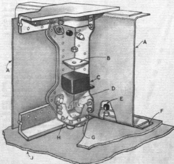
On the left is a detail of the rubber-block internal sealing employed at a typical corner joint of the wing tankage. A, tank wall; B, pressure plate; C, moulded Hycar block; D, tapered faces to be sealed; E, Hycar sealing plug; F, packing strip; G, butt gap sealed by plug; H, retaining welded-steel box for Hycar block, the latter removed by unbolting.
