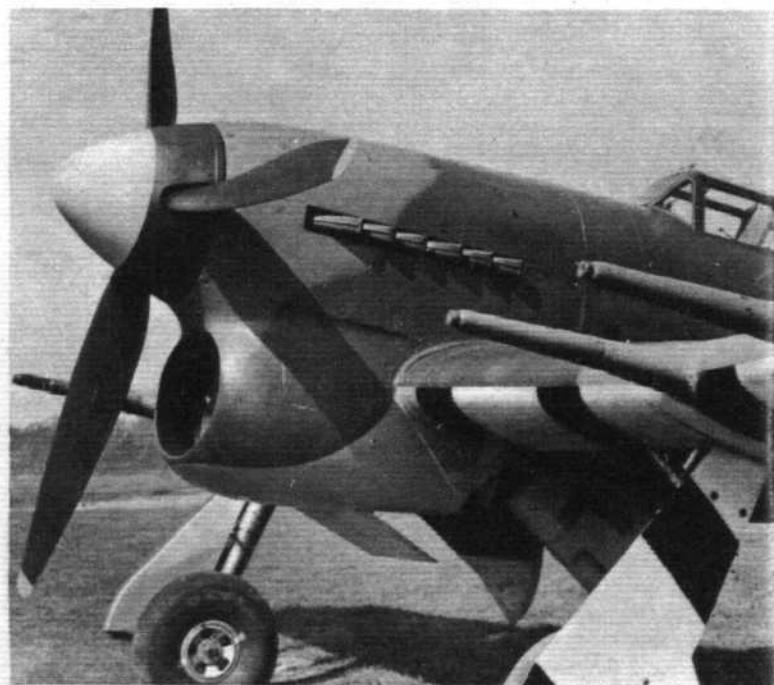
Sabre installation in Hawker Typhoon.
