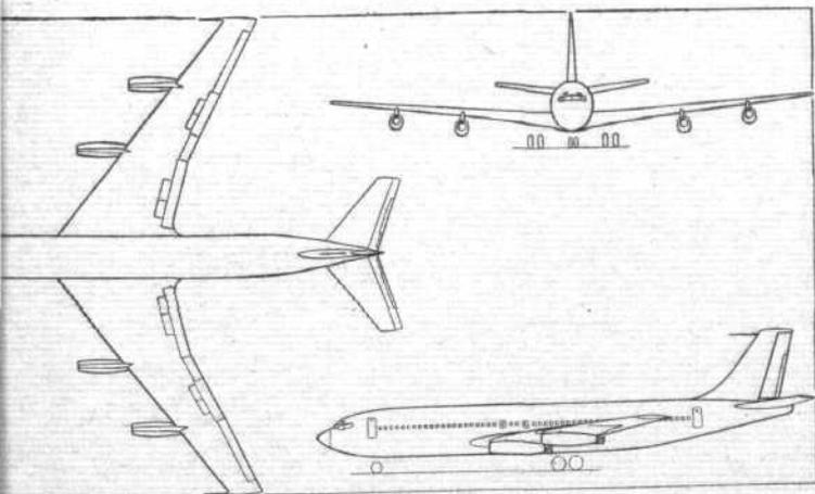
main and inboard sections form a common structure with the fuselage and are not detachable. The primary structure consists of two widely spaced spars forming a box with rib-supported upper and lower skins stiffened with extruded stringers. The spars largely carry the shear loads while bending loads are reacted in the skins.
