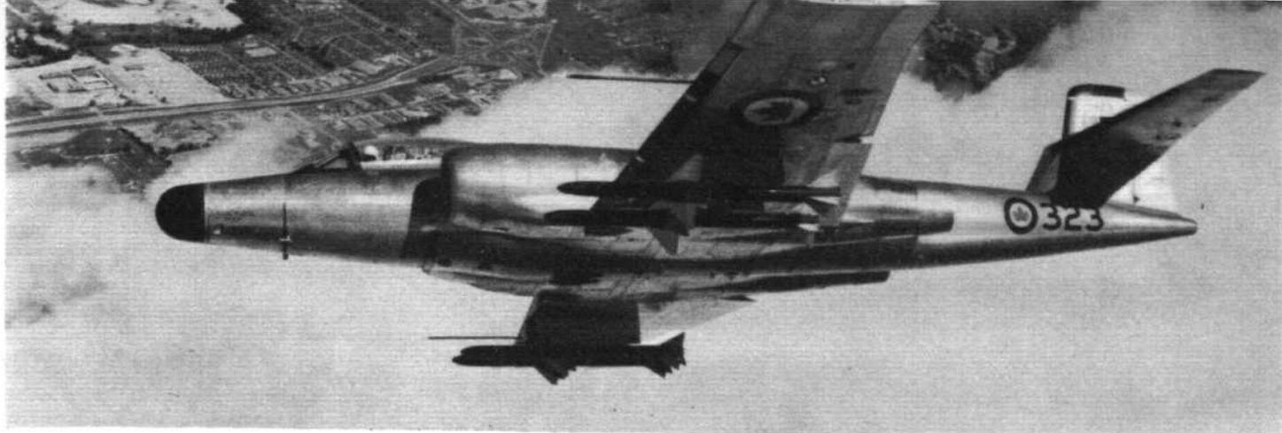
An Avro CF-100 Mk 5M equipped with dummy Sparrow 2 missiles and re-heat version of the Orenda 11.
