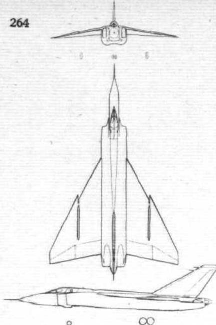
**CF-105 Arrow 1:** Powerplant, 2 P. and W. J75; span, 50ft; length, 77ft 9½in; gross wt, over 65,000 lb; max. speed, over M=2.
