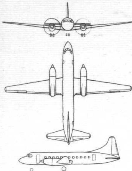
**CL-66:** Powerplant, 2 Napier Eland; span, 105ft 4in; length, 81ft 6in; gross weight, 53,200 lb; cruising speed, 325 m.p.h.
