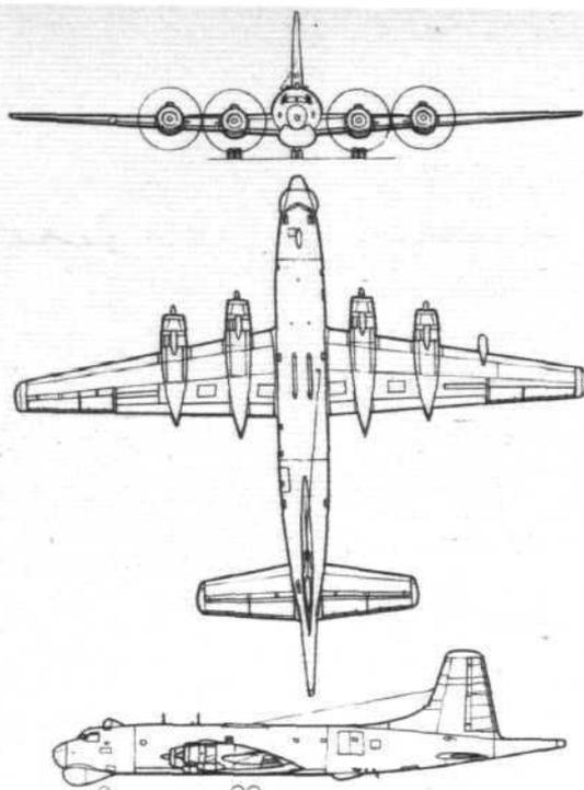
**CL-28 Argus:** Powerplant, 4 Wright Turbo-Compound; span, 142ft 3½in; length, 128ft 3in; gross weight, 148,000 lb; cruising speed, 230 m.p.h.
