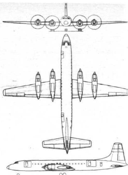
**CL-44:** Powerplant, 4 Rolls-Royce Tyne; span, 142ft 3½in; length, 136ft 9in; gross weight, 205,000 lb; cruising speed, 368-375 m.p.h.
