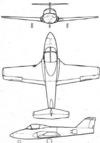
**CL-41:** Powerplant, Fairchild J83; span 36ft 4in; length, 32ft; gross weight, 6,500 lb; max. speed, 445 m.p.h.
