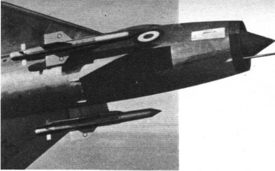
*D.H. Propellers Firestreaks on an English Electric P.1B.*
