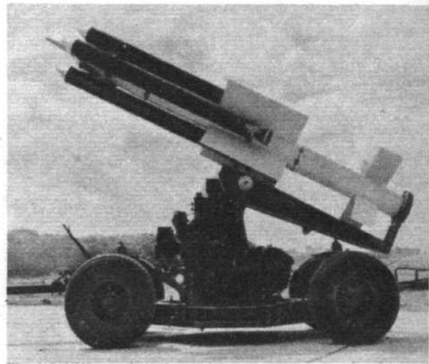
*Above, an Armstrong Whitworth Seaslug ship-to-air missile on a wheeled transporter; below, loading a Bristol Bloodhound ground-to-air weapon into a Blackburn Beverley.*
