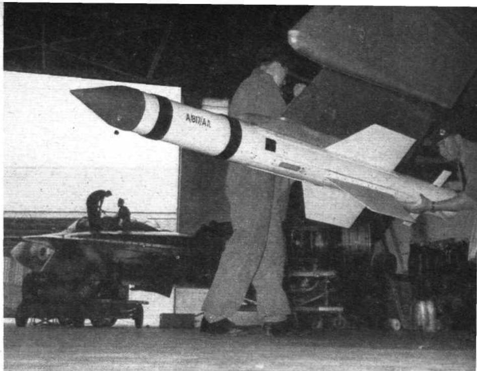
Standard air-to-air missile for the fighter squadrons of the R.A.F. and R.N. will be the D.H. Propellers Firestreak. This round, seen under the wing of a Javelin of Fighter Command, has a conical plastic cover protecting its eight-faceted glass nose
