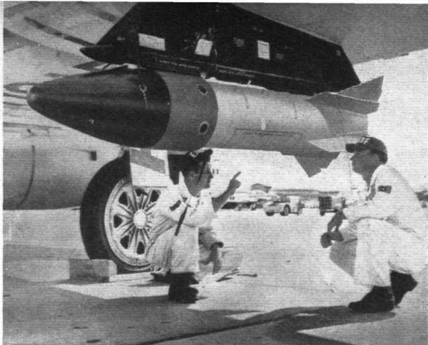
Perhaps the most lethal air-to-air missile in the western world is the nuclear-tipped MB-1 Genie. For more than a year this has been in squadron service with the U.S. Air Force; this one is carried by an F-89J and is illustrated with its stabilizing fins in the extended position
