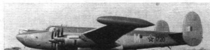
**Avro 496 Shackleton MR.3** (four Rolls-Royce Griffon 57A piston engines of 2,455 h.p. each). Ten-seat maritime-patrol aircraft. Span (over tip tanks), 119ft 10in; length, 92ft 6in; height, 23ft 4in; gross weight, 100,000 lb; normal cruising speed, up to 220 kt; typical cruising range at 1,500ft with full military load, 3,180 n.m.; at a radius of 1,000 n.m. from base the MR.3 can conduct a 9 hr search with radome extended.
