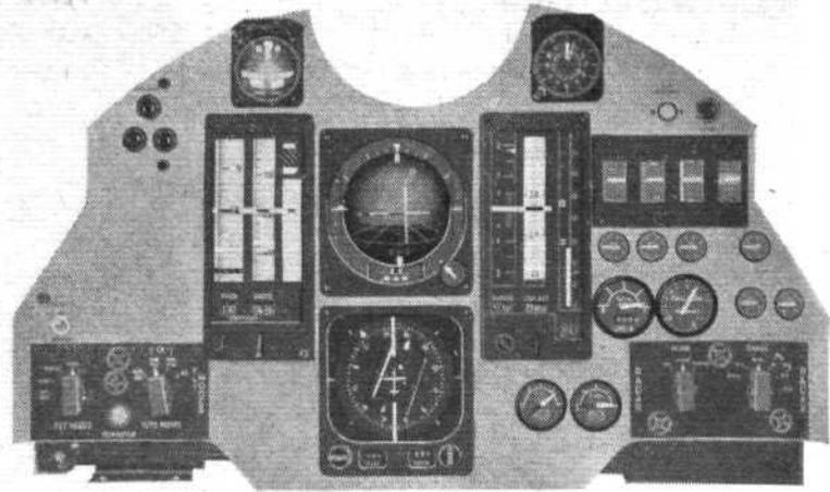
The U.S.A.F. instrument panel to be incorporated in F-106s and F-105s. Plan-position and attitude-command instruments supplied from remote sensors are flanked by tape indicators for speed and height values
