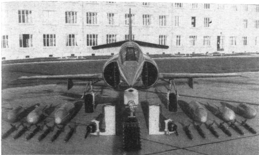
A Dassault Etendard IV surrounded by stores, including the two 30 mm cannon and the rocket pack which can be accommodated alternatively in a fuselage bay. The Marine Etendard does not have the low-pressure tyres shown here
