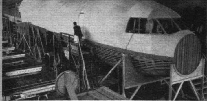
**THIRD DIMENSION** of the VC.10 has now been created by a full scale engineering mock-up of the aircraft at Vickers' Weybridge factory. Thirty-five have been ordered by B.O.A.C. for delivery in 1963-64
