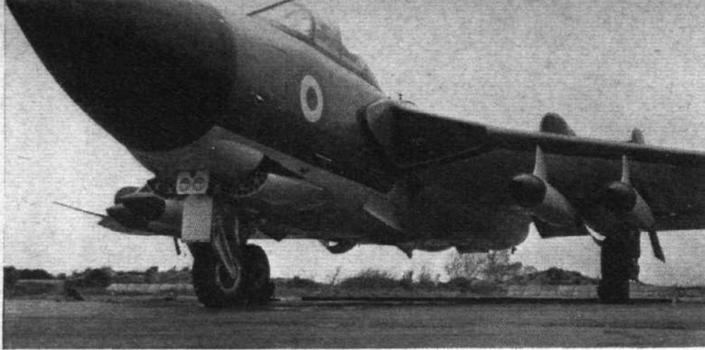
Not fitted with guns, the de Havilland Sea Vixen FAW.1's internal armament comprises hinged packages each housing tubes for 14 spin-stabilized 2in rockets. A further four packs, each of 24 rounds, are here slung from pylons. Made by Microcell, these containers have been proved during high-speed air firing
