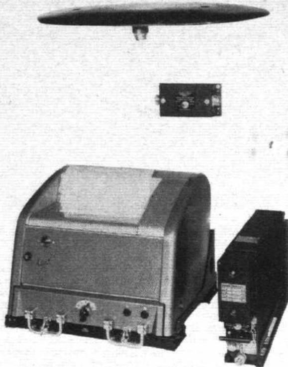
The Marconi AD.308 transistorized H.F. receiver and flush aerial with Creed airborne teleprinter for airline use
