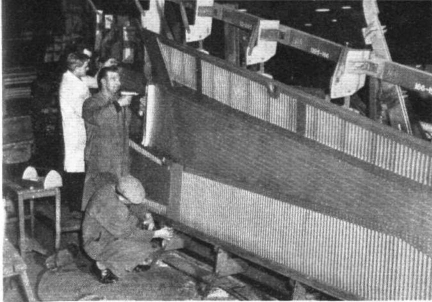
In the text the construction of the Victor is dealt with at length. The photograph on the left depicts the assembly of a complete tailplane, the "grain" directions of the various corrugated panels being clearly visible (also illustrated in a drawing overleaf)
