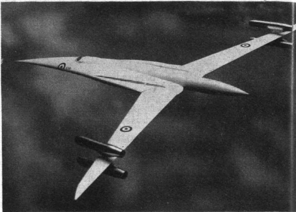
603. The production Wasp is a larger aircraft, powered by a Blackburn A.129 rated at 970 s.h.p. and with a gross weight of 5,000lb. It will be fitted with comprehensive equipment, including autostabilization, for deck-operation in all weathers.
