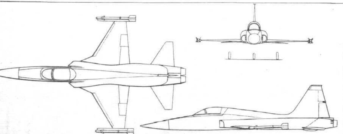
This drawing depicts the final N-156F design. The following data apply: engines, two GE J85-5; span, 25ft 3in; length, 45ft 1in; height, 13ft 1in; tailplane span, 15ft 4in; wheelbase, 11ft 2in; track, 10ft 9in; gross weight, 12,190lb (overload limit with external stores, 16,300lb); max speed, in excess of M2 (1,320 m.p.h.); range, more than 2,000 miles with external tanks; landing distance from 50ft, approximately 3,000ft
