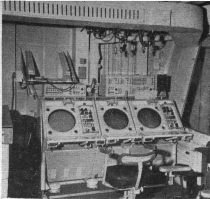
The command staff position in the upper operations room of the carrier defence system using the type 984 radar in HMS "Hermes." The system was produced by Pye. Both hand and foot-operated controls are fitted to the consoles and an electronic "tote board" is used in the main plotting centre
