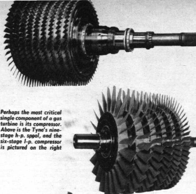
Perhaps the most critical single component of a gas turbine is its compressor. Above is the Tyne's nine-stage h-p. spool, and the six-stage l-p. compressor is pictured on the right
