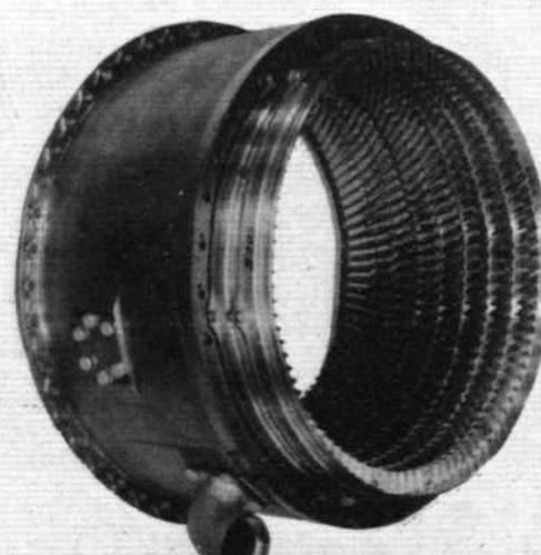
Towards the end of the opposite page it is pointed out that the h-p. compressor stators are carried in steel rings lying inside the stress-carrying outer shell. Both shell and rings are here evident
