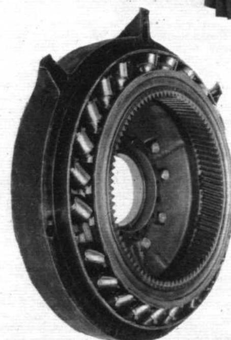
Housed within a casing of magnesium alloy, the reduction gear annulus is surrounded by 24 torque-meter dashpot cylinders. The operation of the torque-meter, and of the automatic drag-limiting system, is described on page 566
