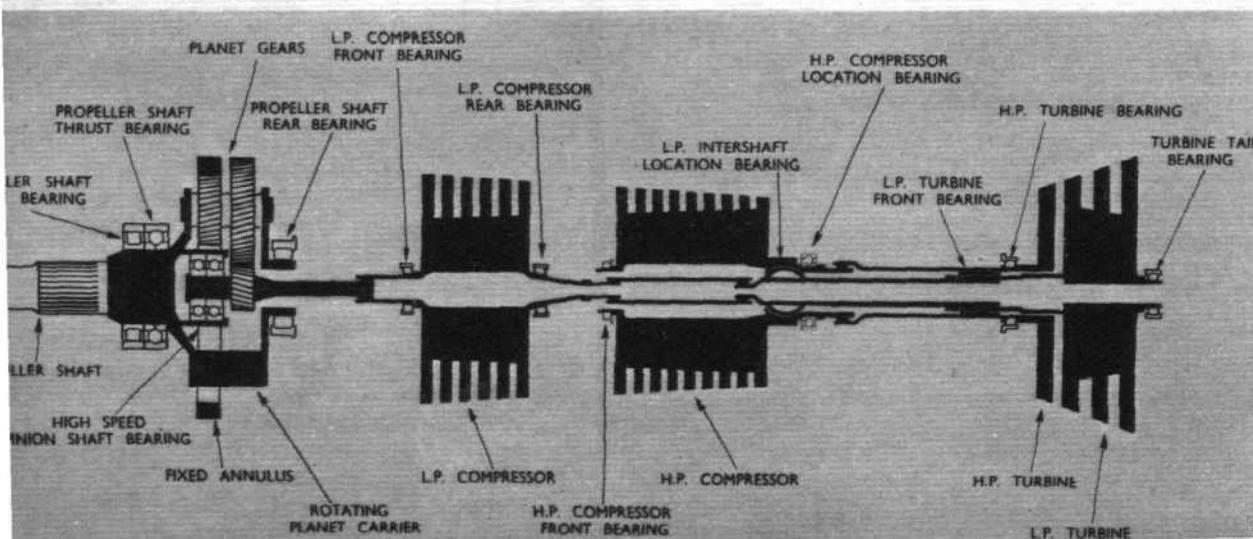
This diagram, which is not strictly to scale, clarifies the basic geometry of the main rotating assemblies. The low-pressure intershaft bearing is shown as a spherical pattern; in fact this is now a ball race, as explained on page 564
