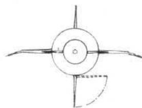
*Dimensions of the Avro Blue Steel Mk 1 include: overall length, 35ft; foreplane span, 6ft 6in; wing span, 13ft; distance from fuselage to start of anhedral, 4ft 10in; fuselage diameter, 4ft 2in; distance from fuselage axis to fin tips, 4ft 6in (upper) and 5ft 4in (lower, extended)*
