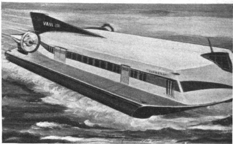
**HOVERCRAFTSMANSHIP:** (Left) Vickers' high-speed hovercraft launch and trials vehicle with an operating payload of up to 4,000lb dependent on powerplant installation. (Right) Proposal for a hovercraft of over 70 tons to operate as a passenger or freight vehicle. A payload of 250 passengers or 25 tons of freight would be carried at 80kt
