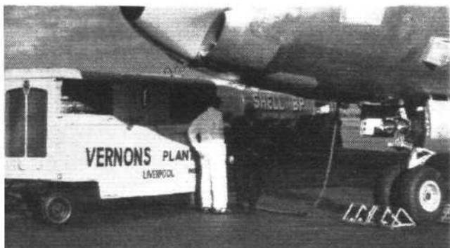
*Vernons 60kVA/12kW ground power unit (AEC diesel engine) in MoA service at Prestwick*
