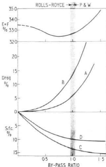
*Curves, plotted against by-pass ratio, of engine+fuel weight for a 1,000 n.m. stage (expressed as percentage of aircraft gross weight), increase in total engine drag (A), increase in total pod drag (B), and reduction in s.f.c. allowing for (C) accessories and air bleed and (D) for increasing pod drag also. As indicated, Rolls-Royce and Pratt and Whitney are both approaching a by-pass ratio of unity, one from below and the other from above*
