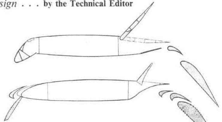
*In their search for greater maximum lift coefficients de Havilland have for the Trident adopted a hinged leading edge, double-slotted flap and upper-surface brake (top). For the 727, Boeing have chosen slats outboard, leading-edge flaps inboard, triple-slotted flaps and spoilers*
