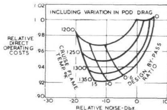
Fig 3 (left). Variation of direct operating cost and take-off noise with combustion flame temperature and design by-pass ratio
