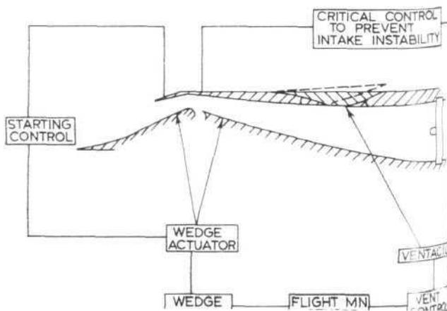
Fig 4 (right). Variable wedge-intake control arrangement for a supersonic aircraft
