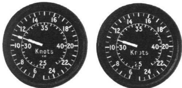
The new Kelvin Hughes twin-pointer a.s.i., showing the two needles aligned for low-speed indication (left) and the short needle indicating 310kt on the inner scale with the long needle trapped so that only its black portions are exposed, and barely visible
