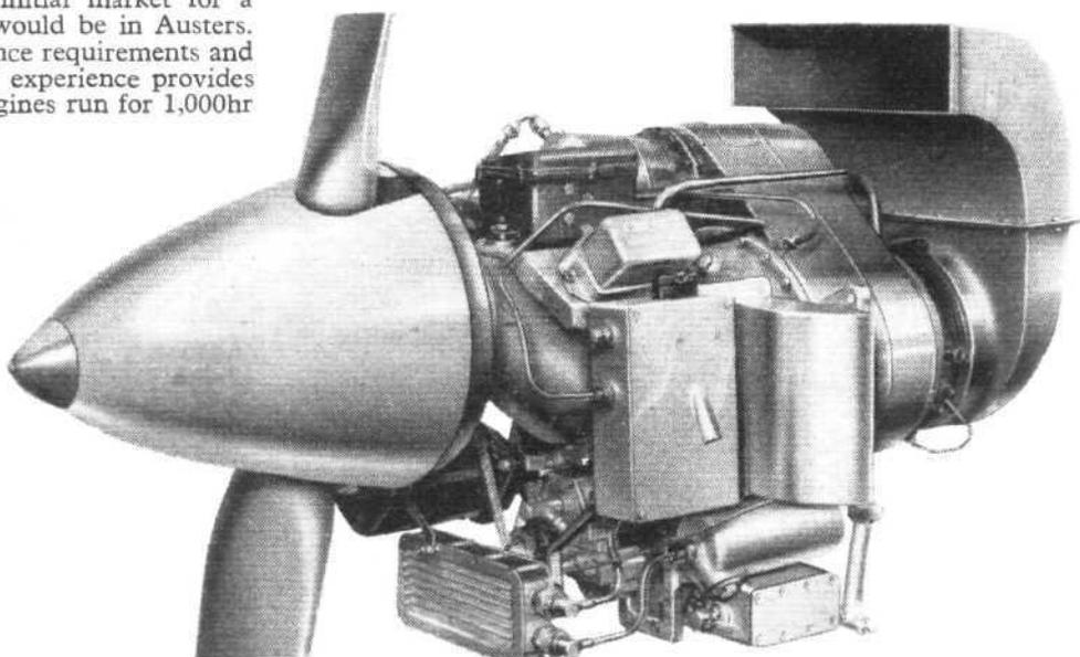
could quite reasonably cope with a Piper Caribbean, although endurance would be somewhat reduced because of higher fuel consumption. The normal optional extra tank of the Caribbean would go some way towards reducing the range penalty. The fuel itself would also be very much cheaper. The engine can indeed accept either kerosine or diesel fuel without any adjustment; and the standard petrol company delivery services would provide fuel anywhere in the country.
