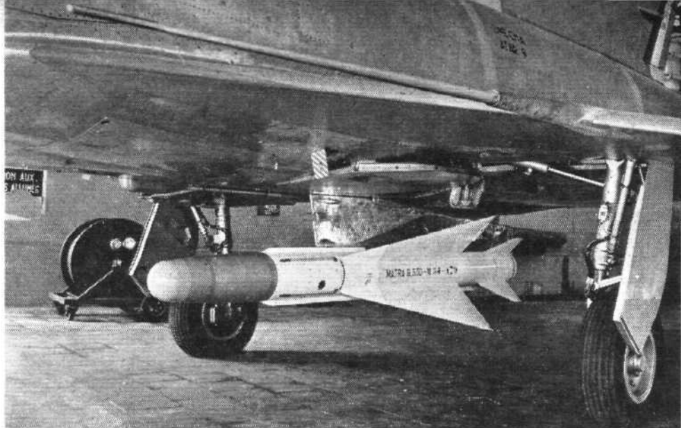
Excellent results are being achieved by the Société Matra with the R.530; it is to be standard armament on the Mirage 3C, an example of which is carrying it in this photograph
