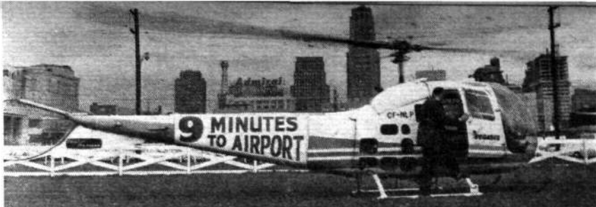
Pegasus Airlifts operates Bell 47J helicopters between Toronto International Airport and heliports in the Toronto area
