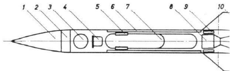
Left, a model of Dornier Type 122 recoverable rocket shown at Stuttgart. Above, typical cross-section of rocket in launch configuration. 1, payload container; 2, electronics; 3, compressed air for actuator; 4, fuel pump system; 5, deployment actuator; 6, Paraglider; 7, fuel tanks; 8, combustion chamber; 9, fin actuator; 10, stabilizing and steering fins
