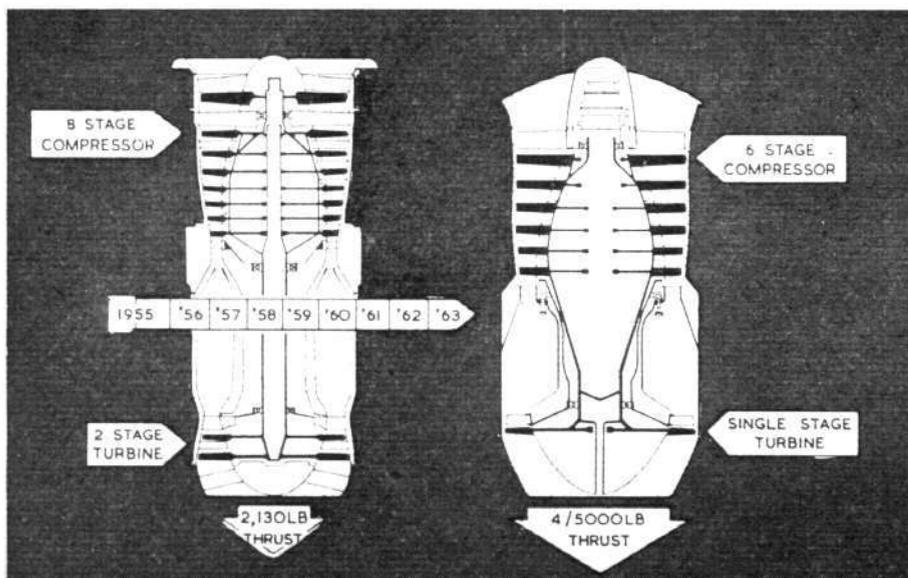
The RB.108 (far left) was the first engine ever designed specifically for the provision of jet lift, and releasable data include: length, 46.5in; diameter, 20.8in; dry weight, 269lb; pressure ratio, 5.25; and thrust/weight ratio, 8:1. The later RB.162 can be seen to be drastically simplified, and its corresponding data are: length, 51.8in; diameter, 25in; dry weight, 275lb; pressure ratio, 4; and thrust/weight ratio, 16:1
