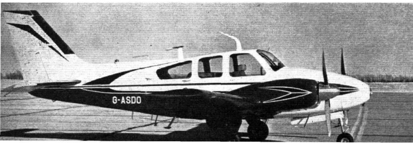
Short Brothers' Baron demonstrator is extensively equipped with full radio, coupled autopilot, de-icing and luxury appointments
