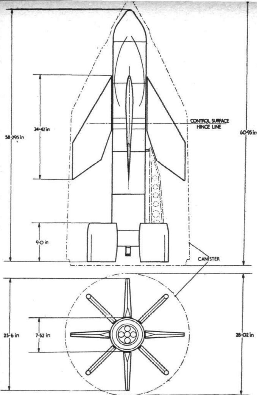
General-arrangement drawing of the Seacat missile
