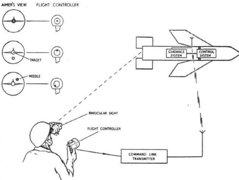
Diagram of the guidance system. Below, wing actuator assembly joints
