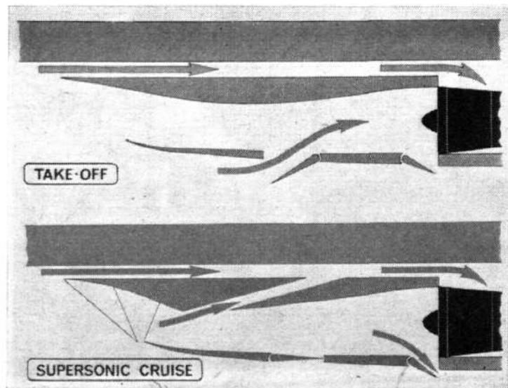
Fig 3 The intake control system. A series of sketches in this journal on June 20 last illustrate the variation in geometry of the intake and the propelling nozzle under all conditions of flight, from sea-level static to supersonic cruise at from 57,000ft to 67,000ft
