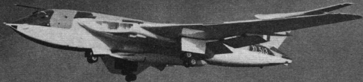
First V-bomber clad in camouflage is this Victor B.2 of 139 (Jamaica) Sqn, landing at Wittering with its limpet-like Blue Steel underneath
