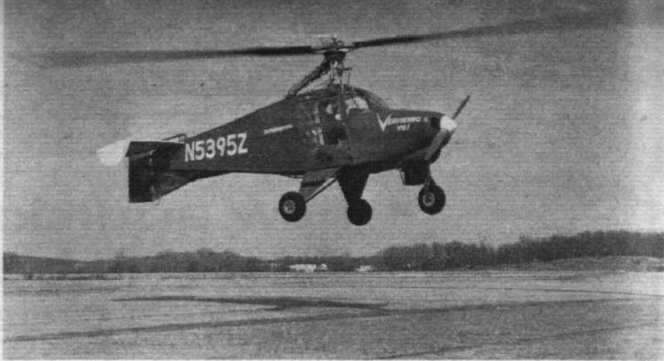
The VG-1 is capable of true helicopter vertical take-off, and of hovering. In this picture the only power is that supplied by the compressed air to the rotor; the nose engine is cut and propeller dead
