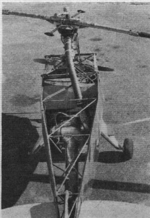
The VG-1 uses a Djinn compressed-air rotor system (far left) raised some 5in to provide rotor clearance over the propeller and tail. The rotor shaft assembly is so designed as not to interfere with cabin area and is neatly mated to the Piper Colt airframe
