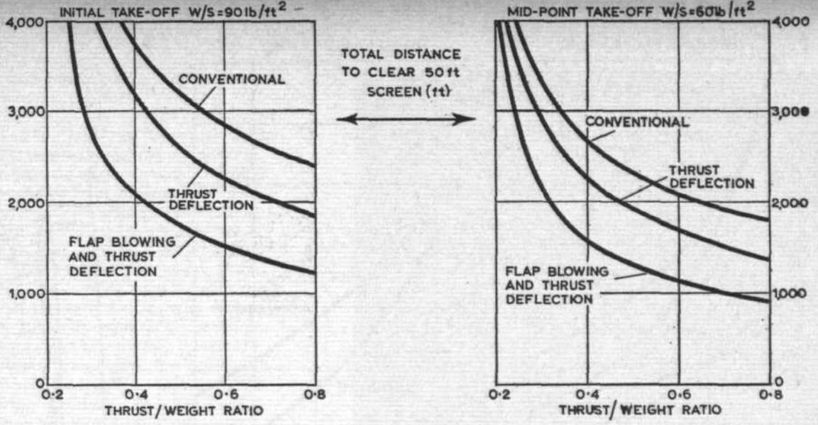
Considerable overloads are possible by accepting field lengths of some 300yd. The take-off technique is to accelerate with nozzles fully aft and then rotate the nozzles to an intermediate position at a speed pre-calculated for a given overload. The time to nozzle-rotating speed—say, 50kt—is extremely short, but the P.1127 has a pre-selector device which enables the correct angle to be applied without the pilot having to look into the cockpit.
