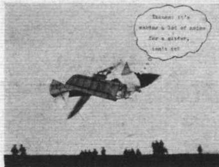
SIR,—I am afraid dear Roger missed the point concerning the break-up of the DH.52 glider (Straight and Level, December 15). What happened was this. The wing had been so lightly built, and was so poor in torsion, that the ailerons functioned only as servo tabs and produced reversed control. "D.H."—remembering wing-warping from ten years previously—decided that, if the glider preferred to wing-warp, why not let it? And so the ailerons were locked and wing-warping controls devised.
