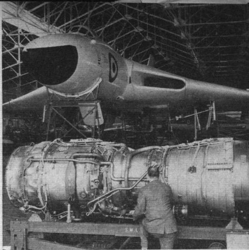
*Transatlantic trio: The Bristol Siddeley Olympus 593 afterburning turbojet and (pictured respectively below) the General Electric GE4 afterburning turbojet and the Pratt & Whitney JTF17A duct-burning turbofan are under development for the West's first generation of supersonic transports—the Olympus for Concorde, and the JTF17A and GE4 for the Boeing 2707 or Lockheed L-2000. Forming the background to the Olympus is its Vulcan test bed*
