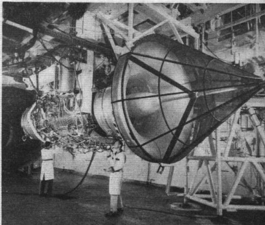
**Bristol Siddeley Olympus 593** single-shaft turbojet with afterburner. Seven-stage axial I-p compressor, seven-stage axial H-p compressor. Cannular straight-through-flow combustion system with eight flame tubes. Single-stage axial H-p turbine, single-stage axial I-p turbine. Air mass flow 450lb/sec. Rating, 35,080lb with afterburner, 32,800lb without. Weight, N.A. Diameter, 47.85in. (See also page 27)
